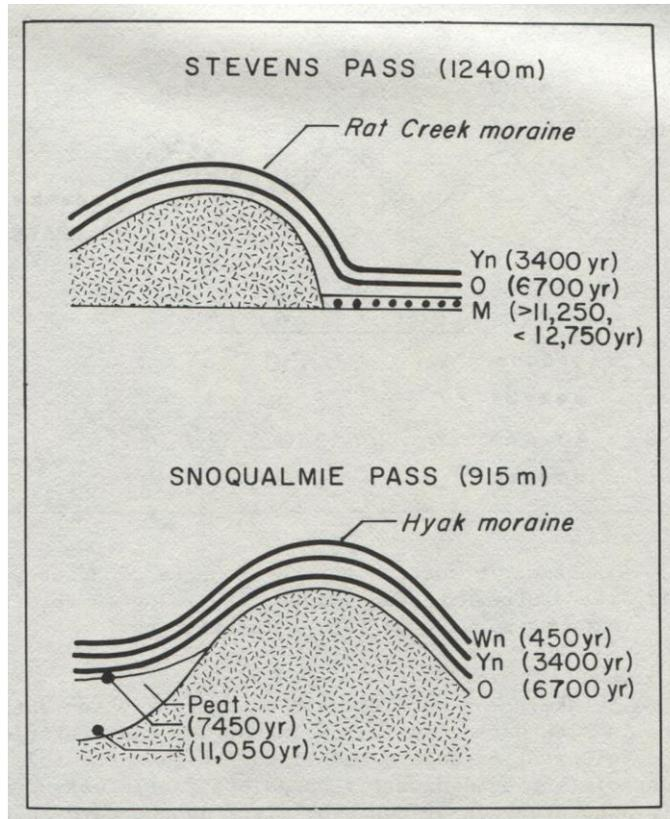
Figure 26. Cross section through Late Pleistocene end moraines at Stevens Pass and Snoqualmie Pass showing relationship of tephra layers. Symbol legend: M = Glacier Peak, O = Mazama, and Yn and Wn = Mt. St. Helens. Source: Porter (1981, p. 147).
